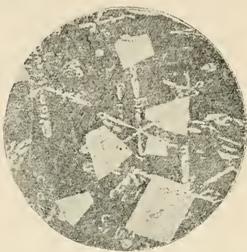
Fig. 8—Alloys of tin, antimony and copper, polished and etched
